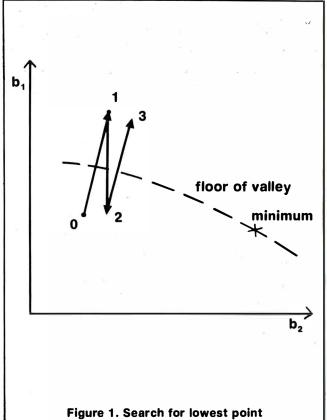
Behavior of steepest descents for the thin, long valley problem. Points 0, 1, 2, and 3 are the initial point and the results of the first three iterations. The movement is largely across the valley rather than toward the minimum point.
